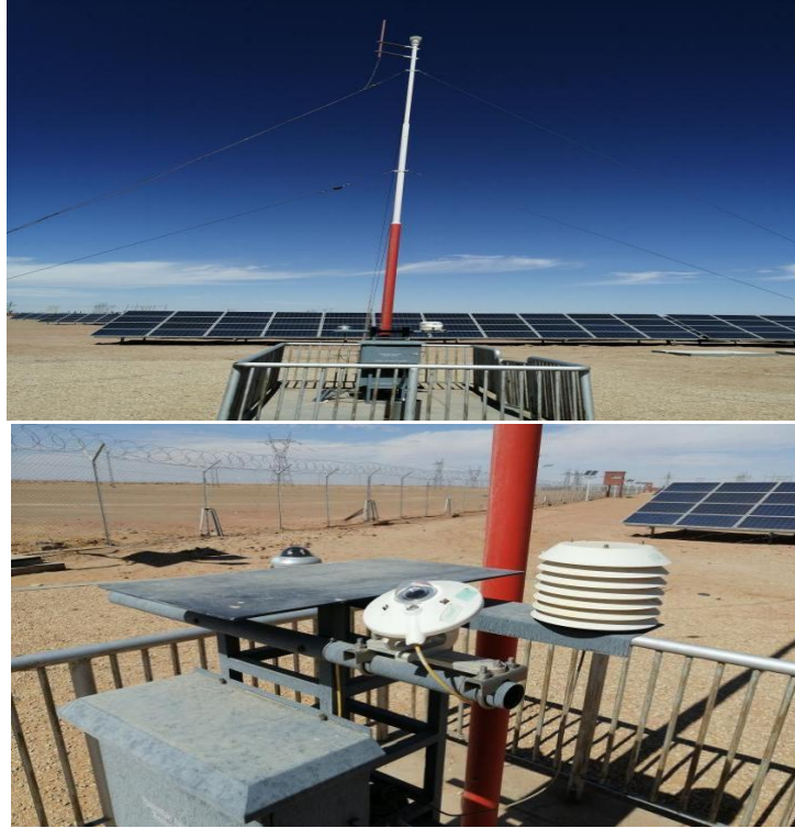
Figure 6. Photograph of meteorological NARI weather station.
