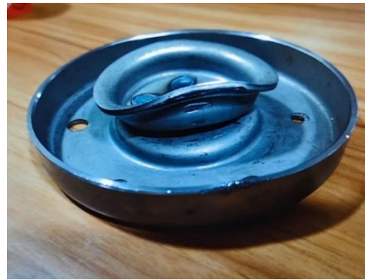
Fig.13 HSLA 355 4 Spot Tensile test welded part
