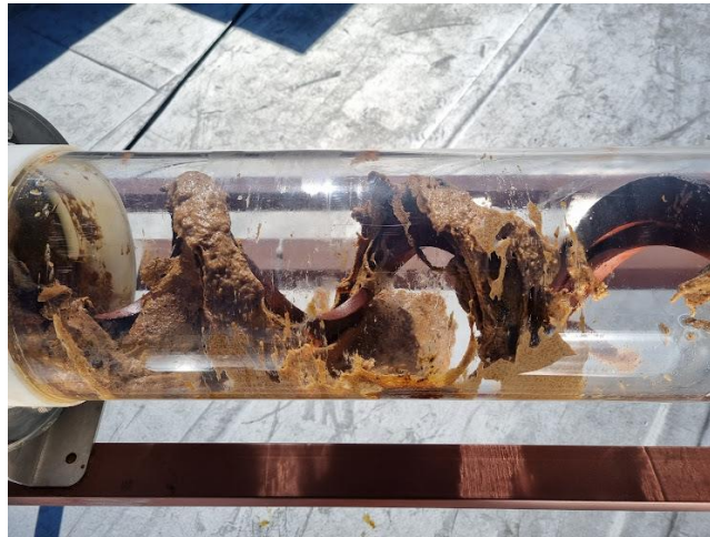
Figure 2. Photograph displaying how synthetic sludge tended to stick to the auger surface
