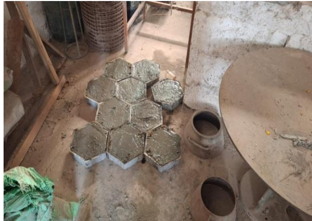
Fig.3.1: Casting of Hexagonal Concrete Paver Blocks Using CETP Sludge
