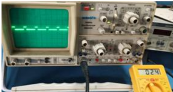
Figure 4.a. Output of KY Converter with Battery Charging
