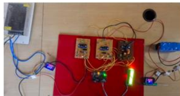
Figure 4.b. Output of Boost Converter with Battery Charging
