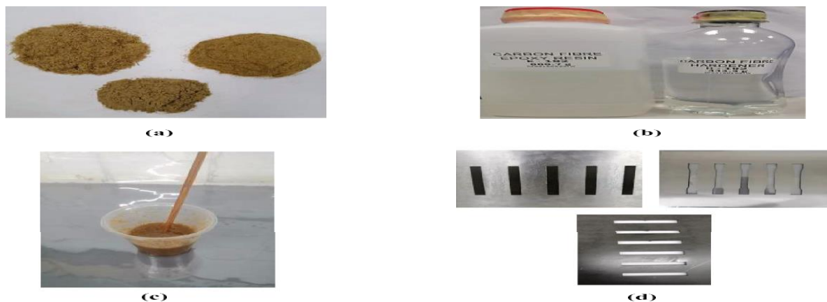
Fig. 1. Photo of (a) bamboo fibers powder (b) epoxy resin and hardener (c) stirring (bamboo fiber), and (d) molding parts of the tensile specimens.
