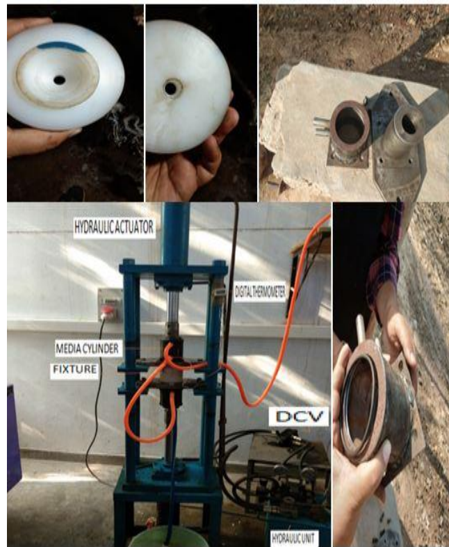
Figure.2 Photograph of Th-AFM setup with nylon fixture
