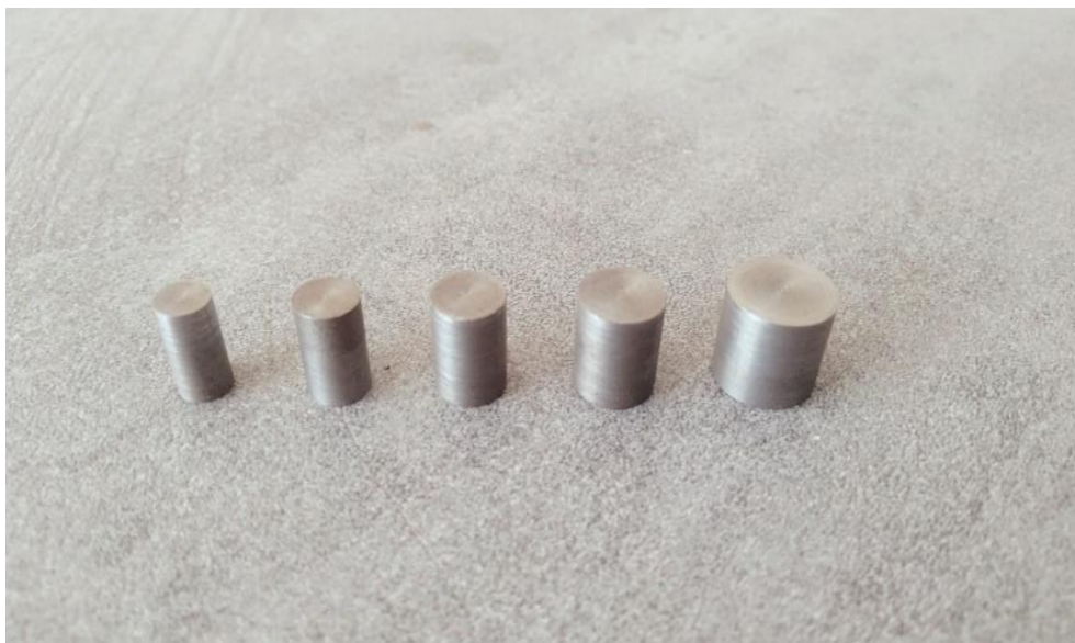
Figure 2.1: Cylindrical specimens of AHSS with varying diameters (5, 6, 7, 8, and 10 mm).
