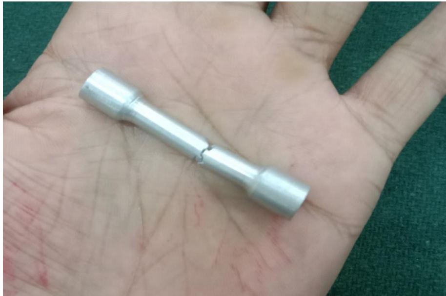
Fig 6: Tensometer specimen prepared in turning operation
