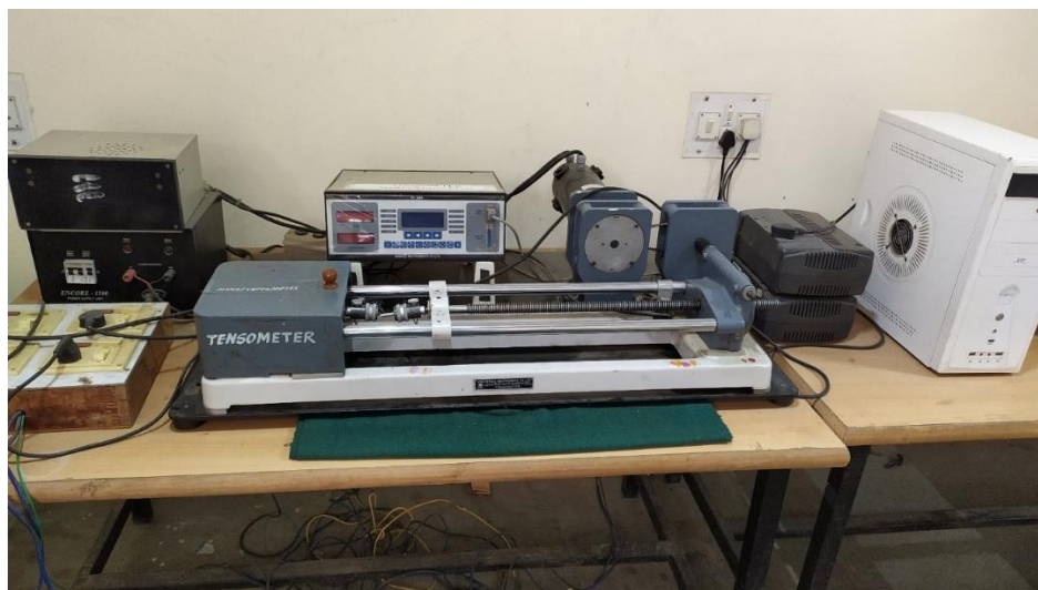
Fig 5: Tensometer setup for finding young's modulus.
