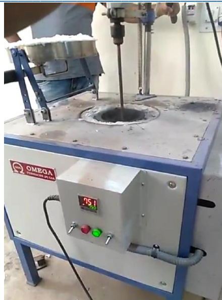
Fig 2: Stirr casting of hybrid composite in a furnace
