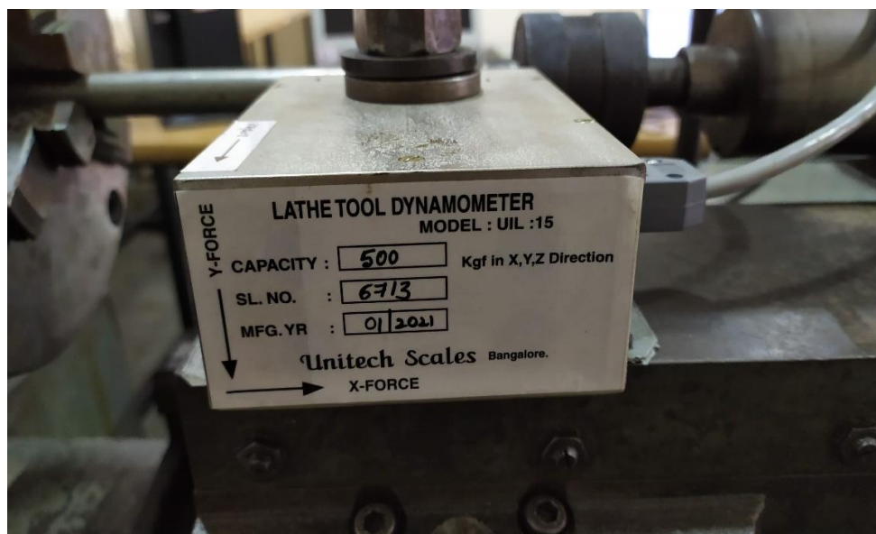
Fig 7: Lathe tool dynamometer setup.
