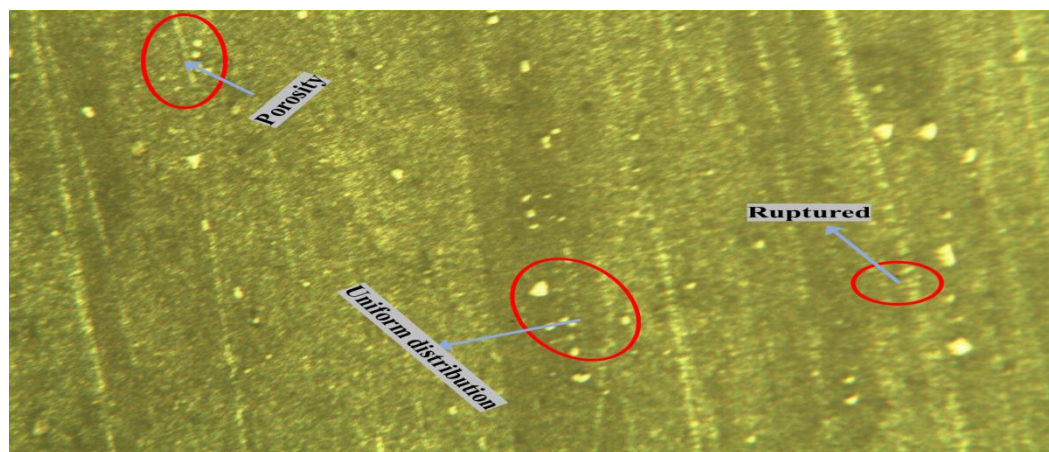
Figure 14. (b) Composite \text{Y}_2\text{O}_3 as-received Scanning Electron Microscope (SEM-SE) picture consumable tool.
