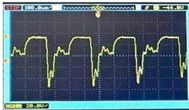
Fig.22. Voltage across Inductor L_s
