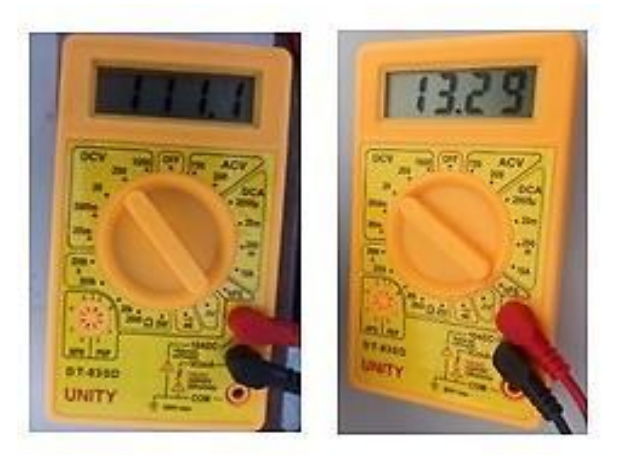
Fig.21. Voltage output in Boost and Buck mode
