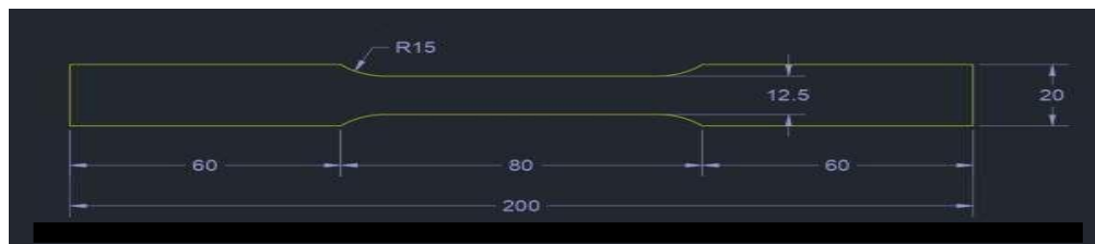
Fig.7 Standard specimens machined for Tension test (all dimensions are in mm)
