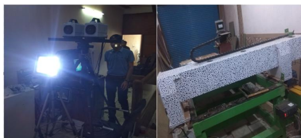
Figure 5: Experimental setup and Speckled Gantry
