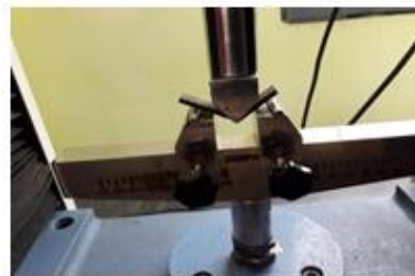
Figure 2.4 UTM with 3-point flexural attachment
