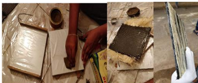
Figure 2.1 Laminate preparations with Compression moulding equipment
