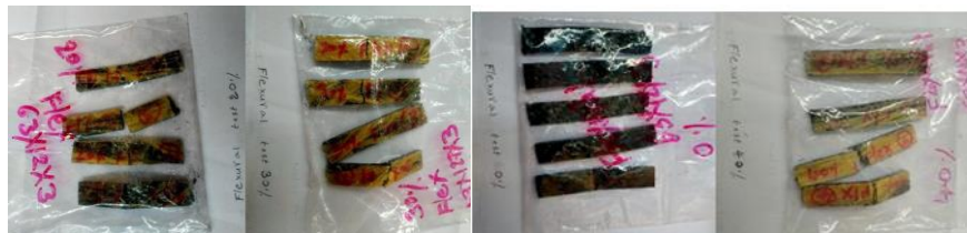
Figure 3.4 Specimens with fibre percentage on flexural strength
