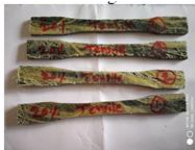
Figure 2.3 Typical tensile test Hybrid composite specimens
