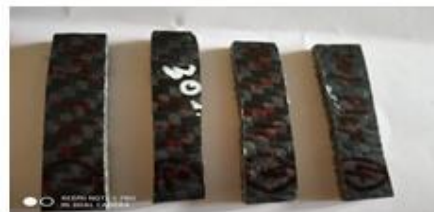
Figure 2.5 Typical flexural test Hybrid Composite specimens
