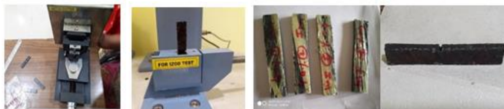
Figure 2.6 Impact testing machine Figure 2.7 Fractured impact test Hybrid Composite specimens
