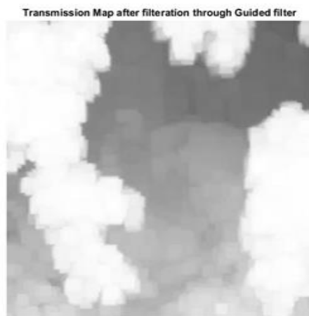
(e)Transmission Map after Filtration through Guided Filter
