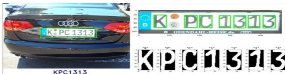
Fig 10: Optical Character Recognition used to detect license plate number
