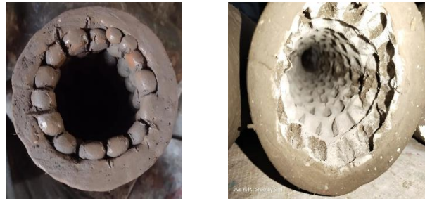
Fig. 1. Test Tubes (a) Protrusion Tube, (b) Dimpled Tube
