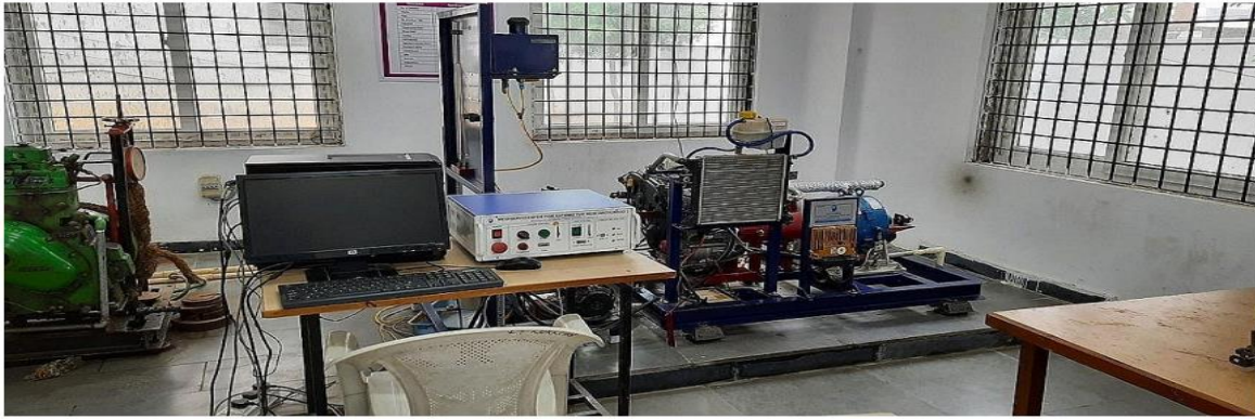
Figure 1. Experimental Setup of CRDI dual fuel Engine
