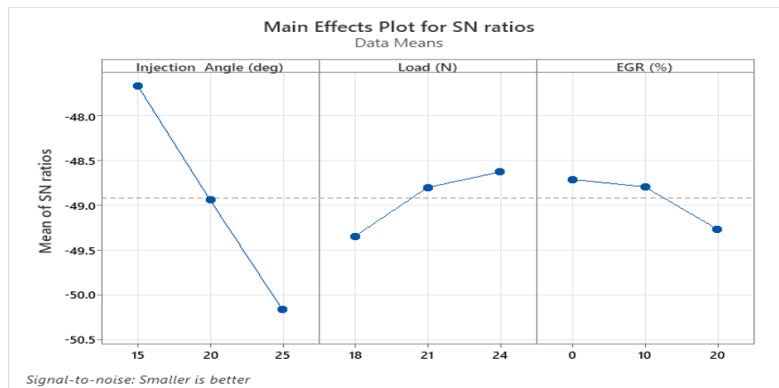
Figure 6. Optimal values of Injection angle, EGR and load for minimizing BSFC
