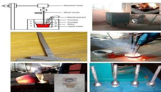
Figure 4. Process of Stir Casting and Al 7178 casted Tools
