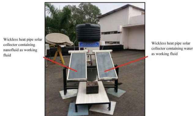
Fig. 1 Wickless Heat Pipes structured solar water heater
