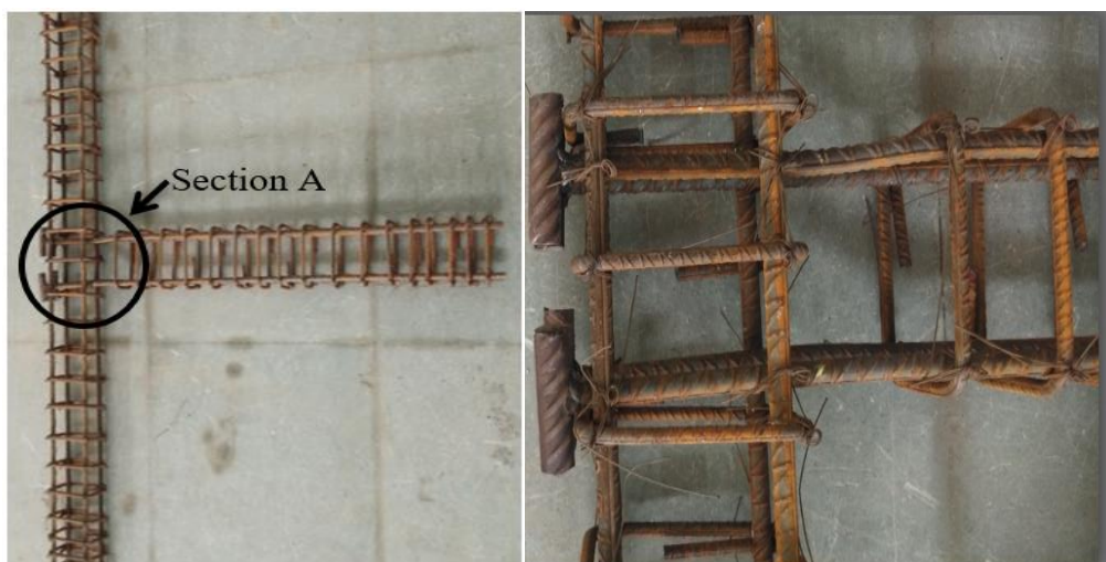
Figure Error! No text of specified style in document..1. Headed bar reinforcement details
