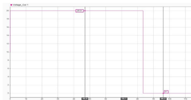
Fig. 15. An Open Circuit Test Conducted on a 20V Channel Input
