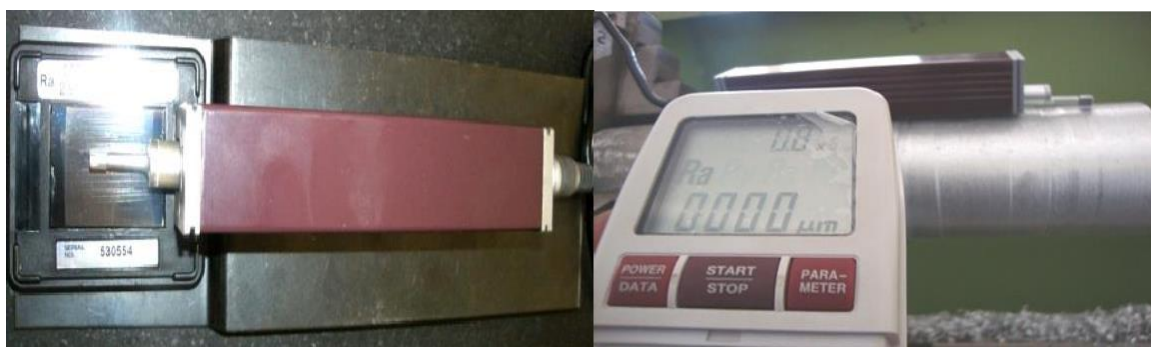
Figure 5: Surface roughness tester used for the experiment
