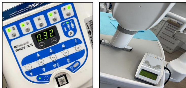
Figure 1: Pictorial representation of incident air kerma ( K_{a,i} ) measurement and parameters sitting in intraoral units.
