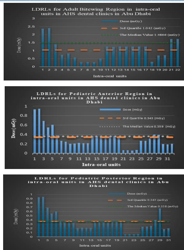
Figure 2: The graphical representation of the determined DRL and the measured K_{a,i} values in dental centers and healthcare clinics in Abu Dhabi
