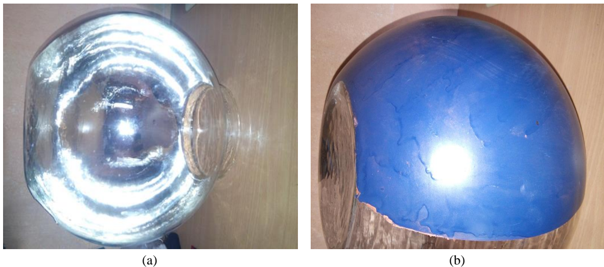
Figure 1: Fabricated hollow spherical collector (a) transparent portion and (b) coated portion
