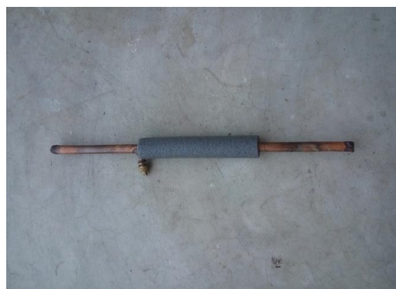
Figure 4: Heat pipe with adiabatic section covered by climaflex
