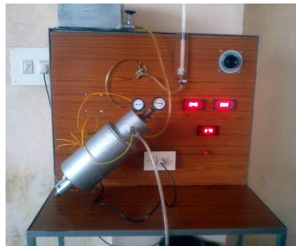
Figure 7: Heat pipe test rig (45° tilt).
