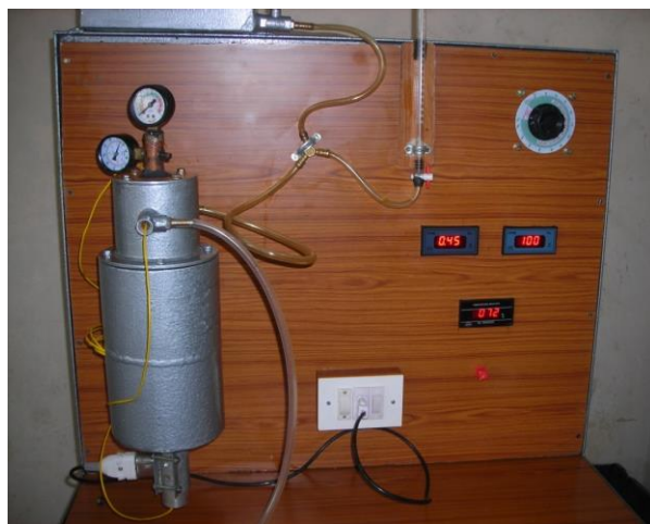
6: Heat pipe test rig (90° tilt).
