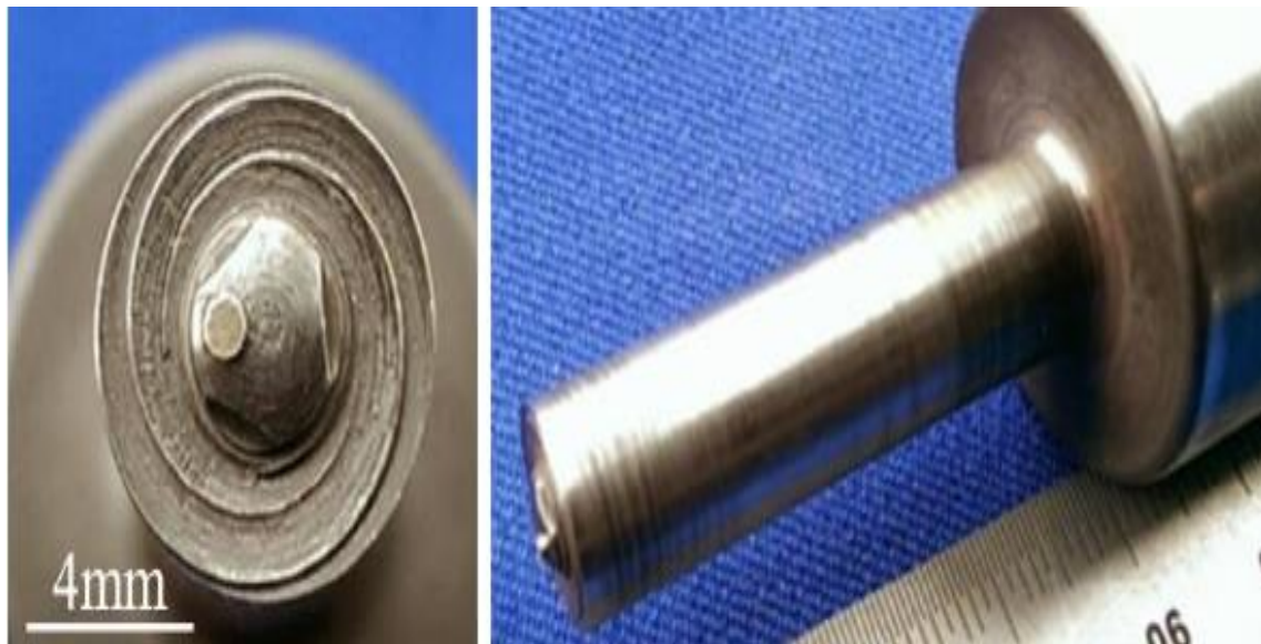
Figure 1.7 Friction stir scribe tool geometry[65]
