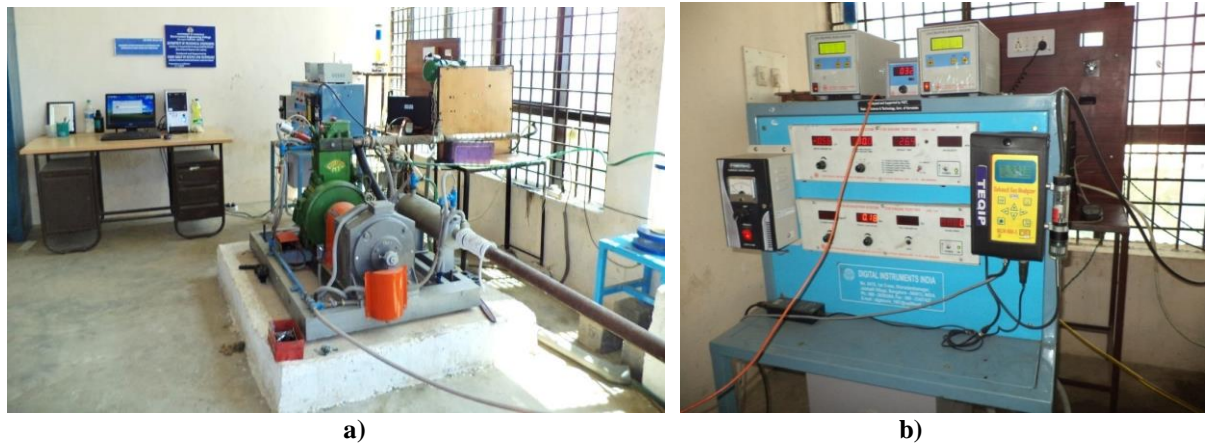
Figure 2: (a) Experimental test rig of computerized diesel engine b) Data acquisition system
