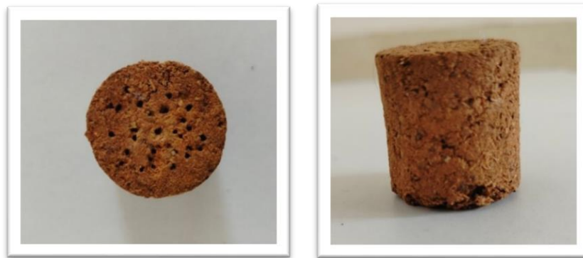
Figure 2. Neem Wood Powder Specimens ( D=35 mm, t=25 mm/ 35 mm).
