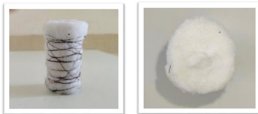
Figure 3. Glass Wool Specimens ( D=35 mm, t=45 mm/ 80 mm).
