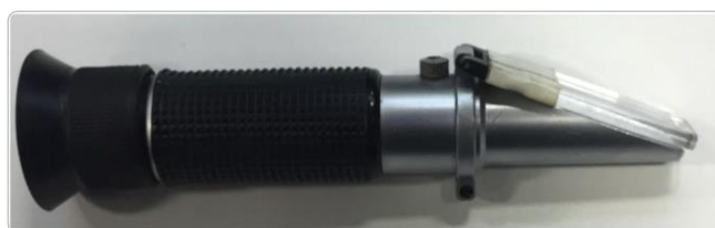
Figure 2. Typical hand refract meter used to measure fluid concentration
