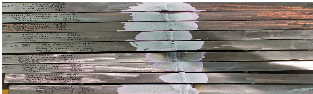
Figure 5.1 Dye penetrant test carried on SS202 specimen
