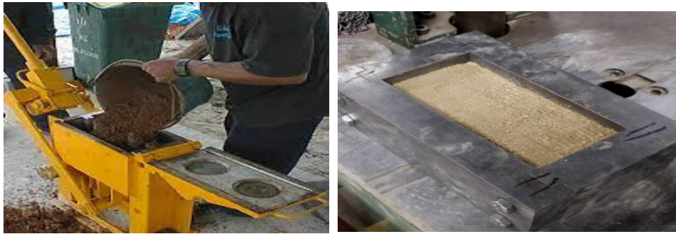
Figure 3: CSEB manufacturing machine
