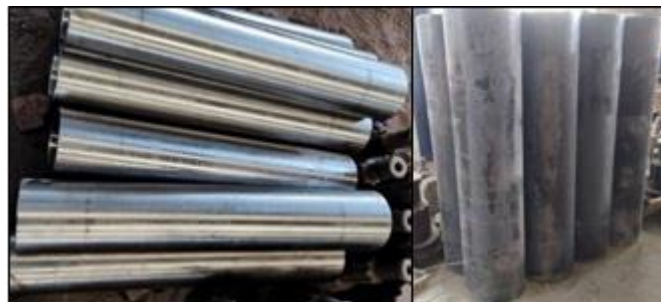
External cylinder before and after heat treatment
