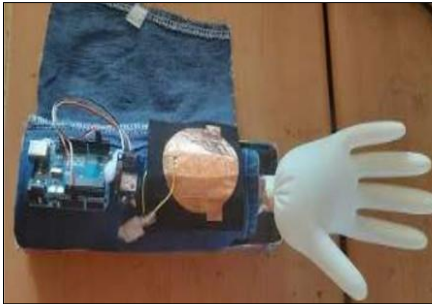
Fig 14: Connection with Arduino board and replacing the antenna of GPS
