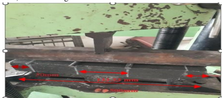
Fig 6 Flexural strength test of concrete
