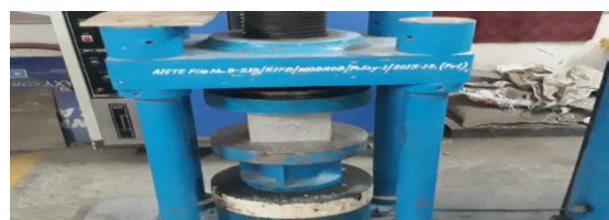
Fig 4:- Compression testing of concrete
