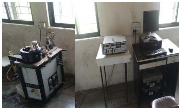
Figure 3. Tribometer experimental test setup
