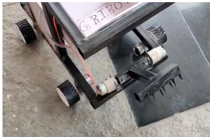
Fig-7: Ploughing mode of the Agriculture Robot
