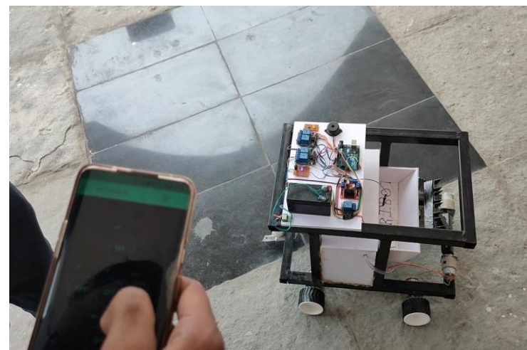
Fig-5: Right Turn mode of the Agriculture Robot
