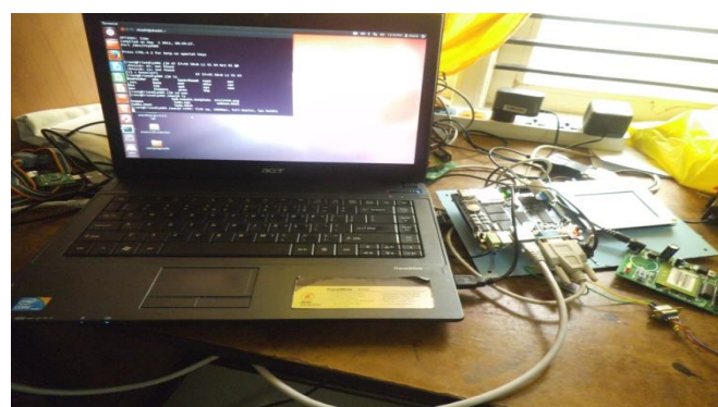
Fig.12. Server side includes mini2440, GSM module and Laptop
