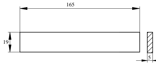
Tensile Test Specimen ( ASTM D - 638)
