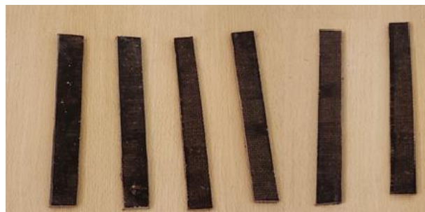
Figure 8. Specimens for Tensile test
