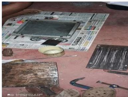
Figure 6. Hand lay-up process
