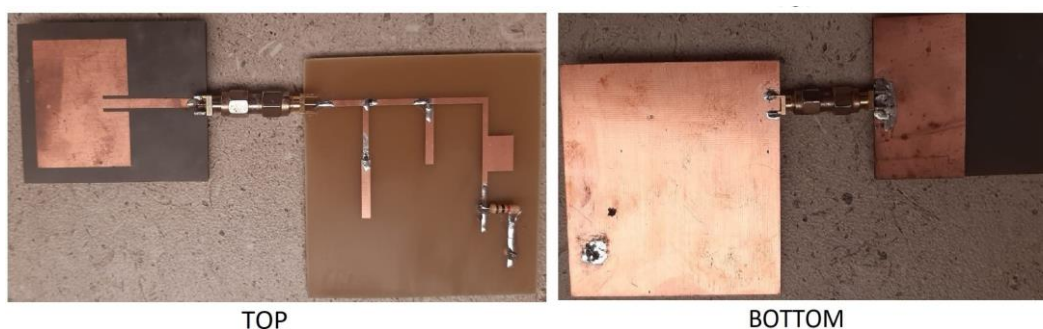
Fig. 7 Fabricated proposed rectenna model.
