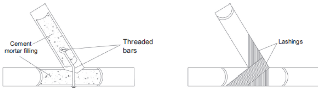
Figure 12. Connection with reinforcing steel and cement filler
