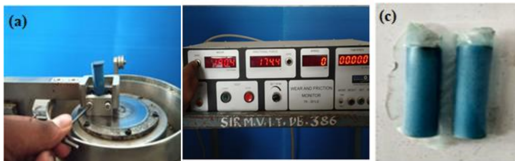
Fig 4: (a) POD wear test machine with sample, (b) wear and friction monitor, (c) Samples
