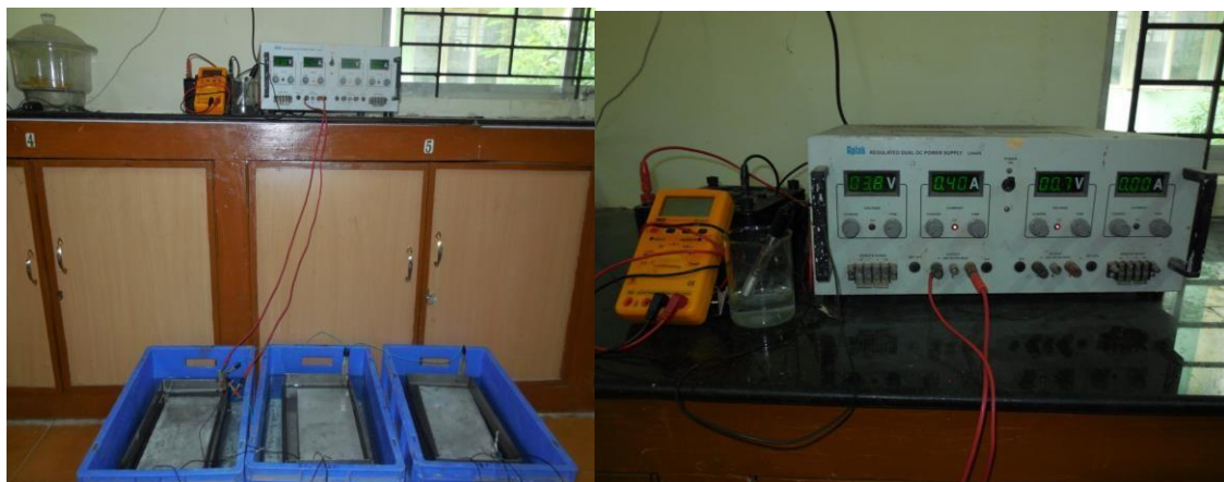
Figure 4– Open Circuit Potential test set-up
