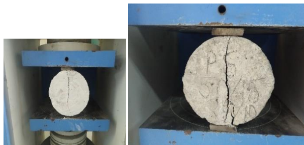
Fig 1.25 Failure Mode of Cylinder Specimens
