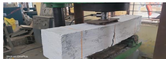
Fig 1.28 Failure Pattern of M60 Beam Specimen under Flexural loading
