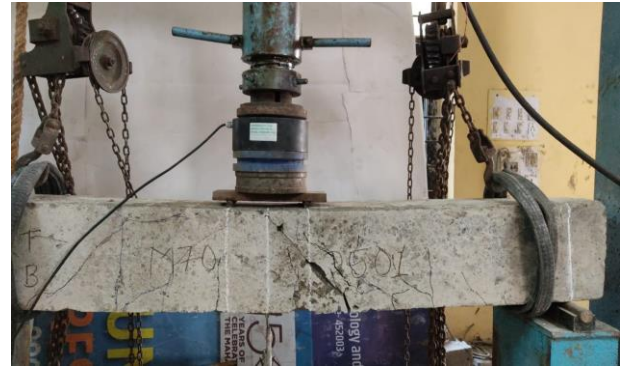
Fig 1.35 Failure Pattern of M75 Beam Specimen under Fatigue loading
