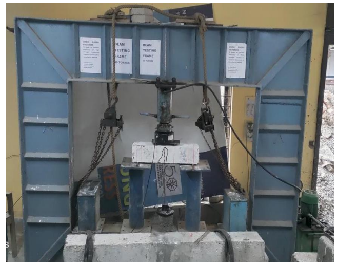
Fig 1.27 Failure Pattern of M45 Beam Specimen under Cyclic loading
