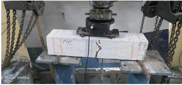
Fig 1.29 Failure Pattern of M60 Beam Specimen under Cyclic loading
