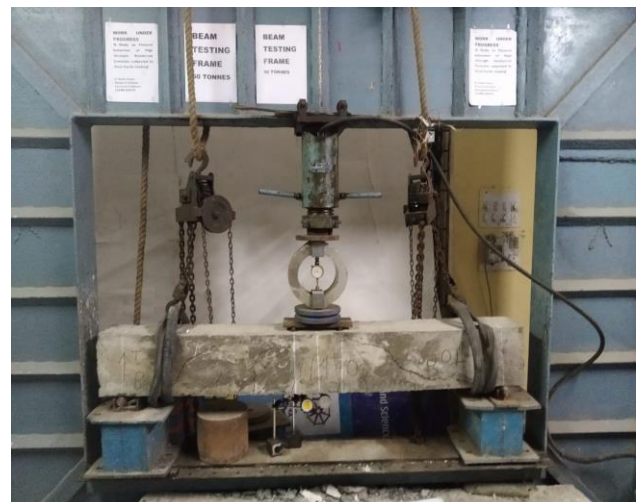
Fig.1.33 Failure Pattern of M75 Beam Specimen under
