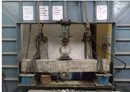
Fig 1.64 Shear Failure Pattern of M75 Beam Specimen under Stability loading
