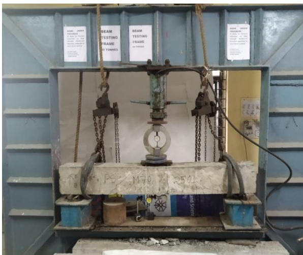
Fig 1.32 Failure Pattern of M75 Beam Specimen under Monotonic loading
