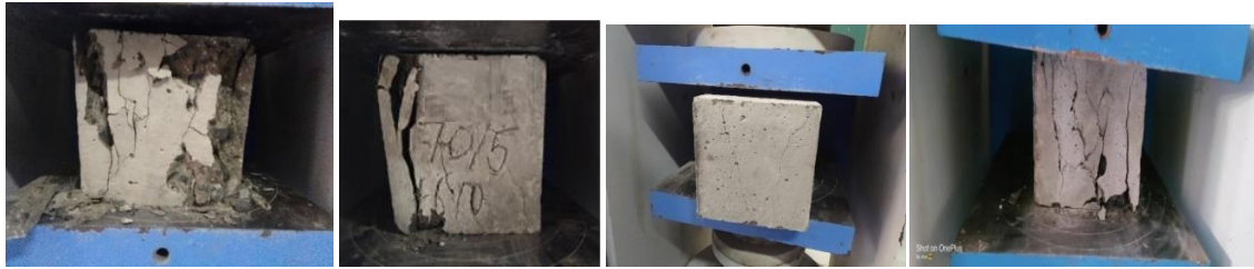
Fig 1.24 Failure Mode of Cube Specimens
