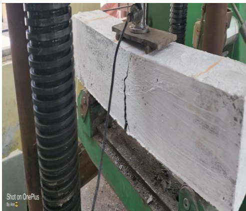
Fig 1.26 Failure Pattern Beam Specimen under Flexural loading (M45)
