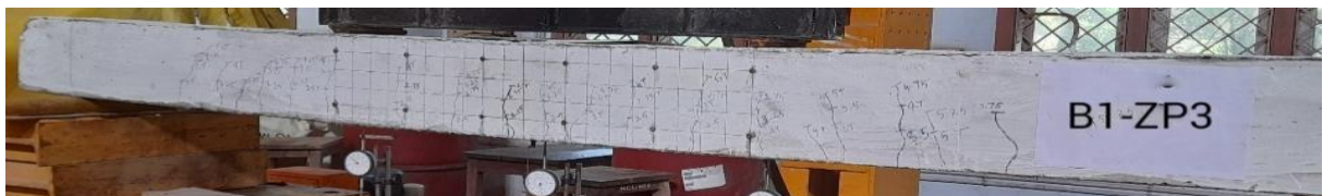
(i) Crack Pattern of B1-ZP3 Beam
