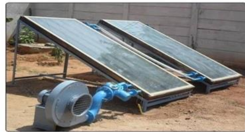
Fig.2 Solar air heater with blower
