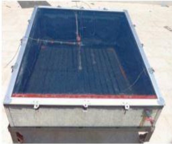
Fig. 4. Finned basin with SSSS [93]
