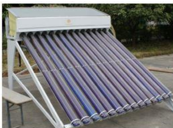
Fig. 2. Vacuum tubes with multi-effect solar still
