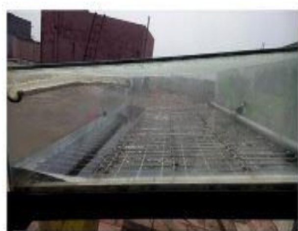
Fig. 5. PV panel in the basin with SSSS [95]
