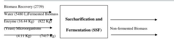
According to above material balance, we get amount of ferment requires for production of 1000 L/Day ethanol. By using this volume we can calculate fermenter thickness, head thickness, inside and outside diameter, Length of fermenter by using design equations. The liquid portion of the slurry has 8-12% ethanol by weight. The whole process requires 48-72 hours. The Batch and Continuous fermentation systems can be used and out of both batch process is more popular.
