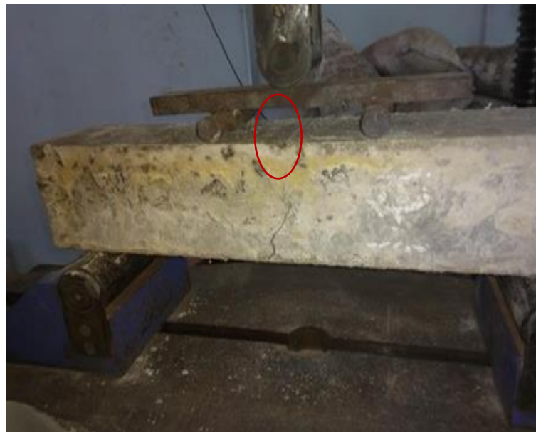
Figure 3: Flexural strength test and crack pattern
