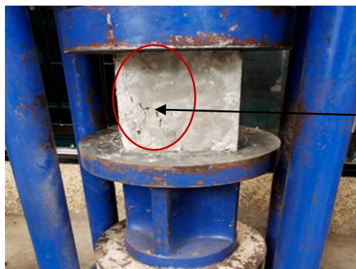
Figure 1: Compressive strength test and crack and crack pattern
