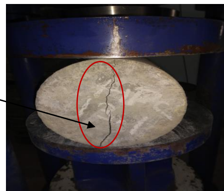
Figure 2: Split tensile strength test pattern
