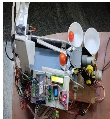
Figure 9. Robotic arm picking the sample on moved on conveyor belt
