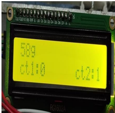
Figure 6. Digital display showing weight and the count value
