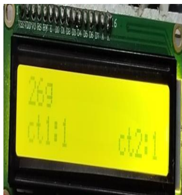
Figure 10. Digital display showing weight and count value
